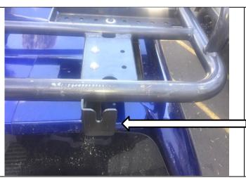
Place the RH & LH mount brackets under the rear of the roof rack accessory mount as shown.
