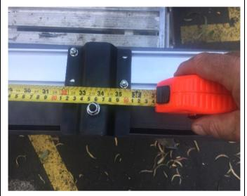
Install awning brackets onto awning and set at the required pitch taken from the previous step.
