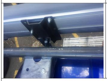
Install 1 M8 flange nut loosely onto each knurled stud.
